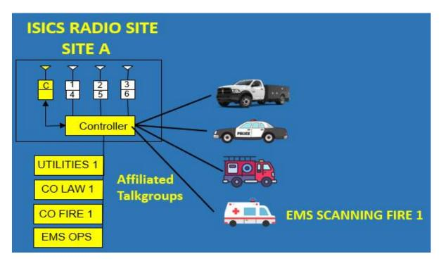
Scanning on a trunked radio system is much different than scanning on a conventional radio system. The trunked system strives to be efficient with all system resources. Channel efficiency means talkgroup audio is broadcast on tower sites where a radio is affiliated.
