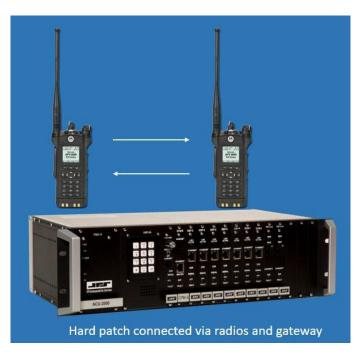
(This diagram shows a hard patch that was initiated at a gateway. In the diagram, two portable radios are connected to the gateway through a wired connection to be able to talk to one another.)
