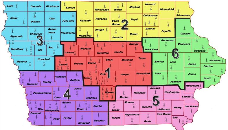
Figure 1. Current map of the ISICS Platform as of December 1, 2022. The tower icons represent ISICS sites. The numbers represent the ISICS operating regions. All sites are networked together with microwave or fiber-optic connections.
